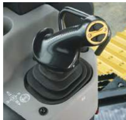
Commandes ergonomiques PCCS (Palm Command Control System)
